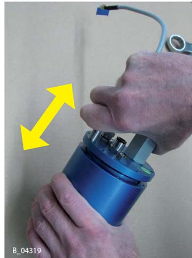
11. Loosen and remove the three generator flange screws.
