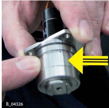
15. Carefully press out generator from the other side (through the screw connection) with a pin.
